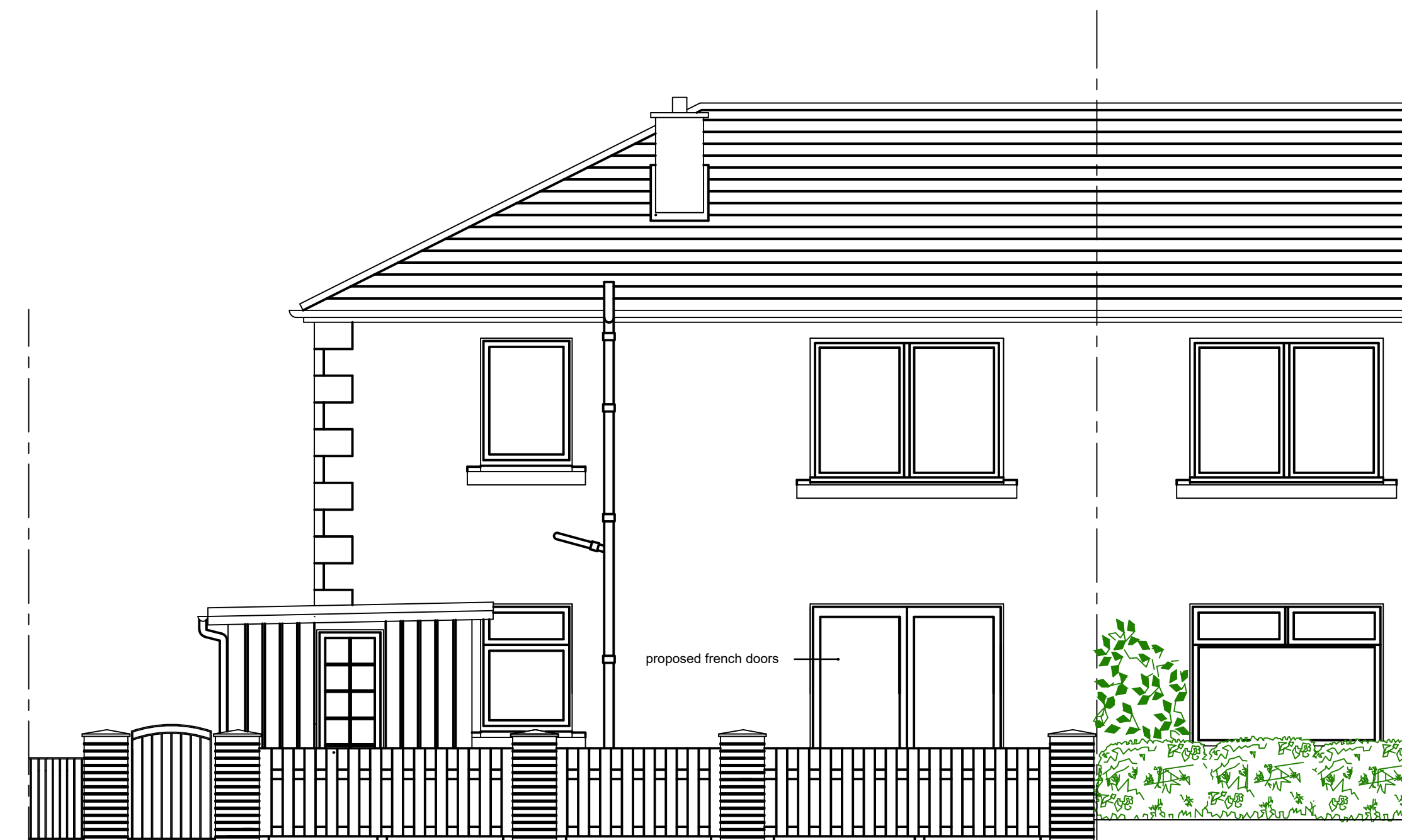
ELEVATION FROM ROAD AS AMENDED
